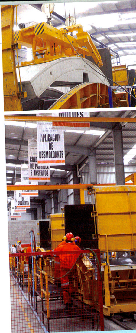
Top: Segments are removed from their moulds using a CBE vacuum beam Above: Casting underway for Mexico City's Emissor Oriente Sewer Project
